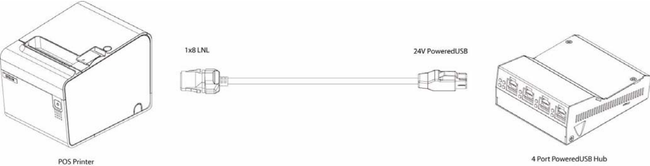
Figure 2-14. Cable, +24V PoweredUSB to 1x8 PoweredUSB
